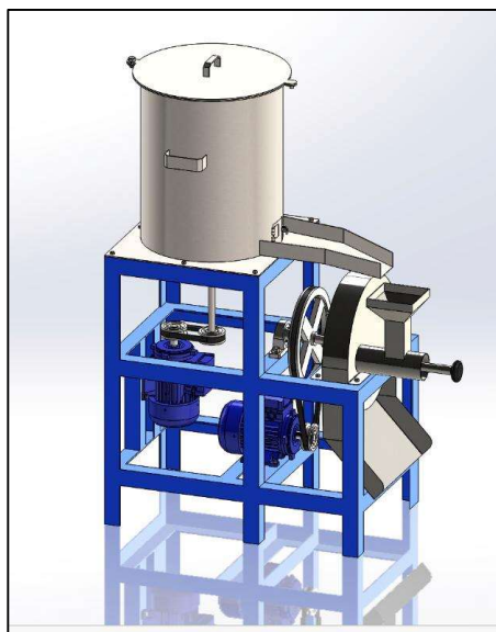
Fig. 2. Design and fabricated prototype of the integrated shallot peeling and slicing machine: (a) three-dimensional design, and (b) fabricated machine.
