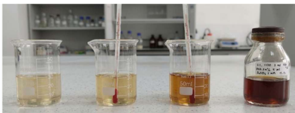
Fig. 4. Visual color change from colorless \text{AgNO}_3 solution to yellowish-brown AgNP colloid during the green synthesis process.
